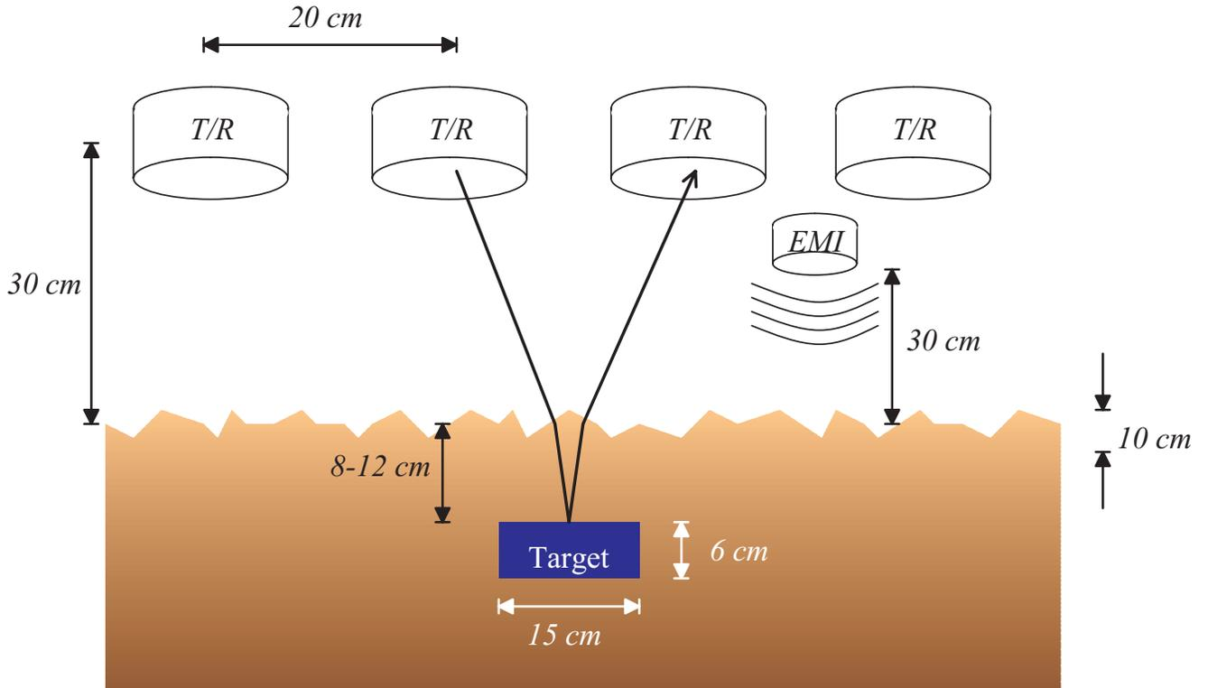
**Figure 2.** Geometry of the sensor/mine configuration
