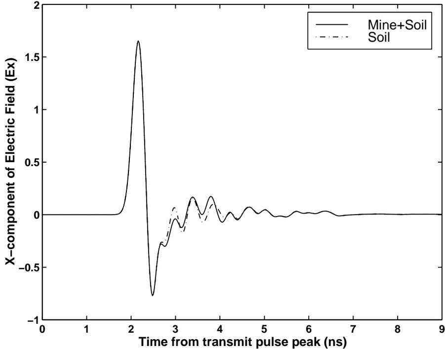
**Figure 3.** Noiseless GPR time traces; transmitter 2, receiver 3
